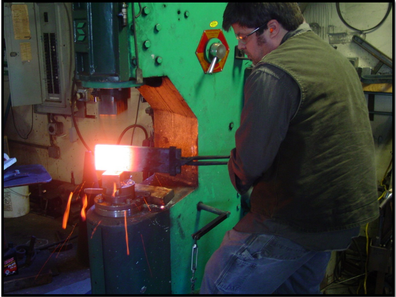
This is a photograph of blacksmith/partner, Timothy Miller (Spirit Ironworks, Inc.) working on the billet that will become one of the decorative urns pictured in the center of the rail. He is using a 135 lb. pneumatic hammer to taper the billet. The steel is heated to approximately 1900°f to make it malleable.
