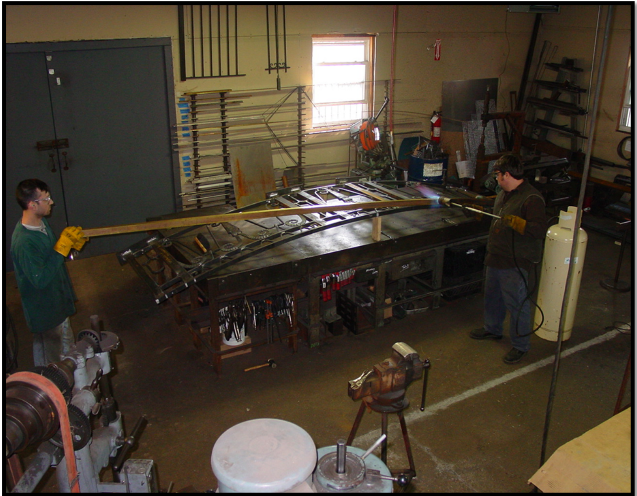
This photograph gives an overhead view of the process. Here you can see one person heating while the other is carefully bending the bronze to match the curve of the railing.
