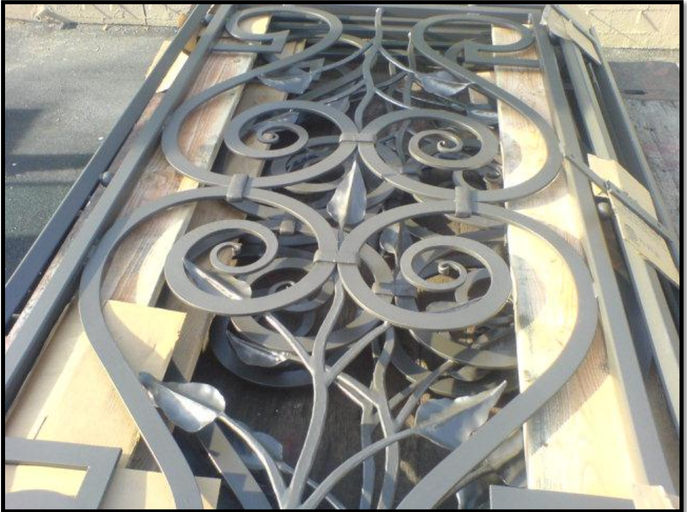
Palletized, packed and powder coated, the pieces are ready for installation.
