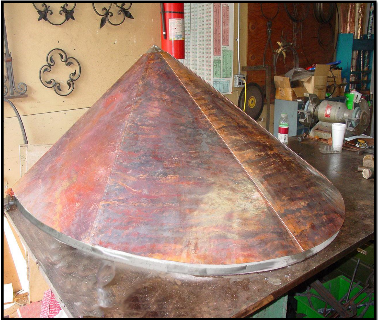
Here is another example of the copper being used as a skin for a stainless steel canopy.
