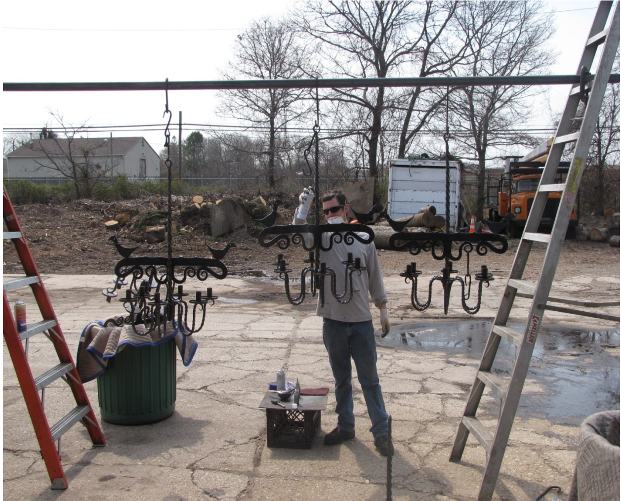
Here is a shot of 3 of the finished chandeliers. They were blackened by hand using a chemical patina and graphite. They were then sealed using a conservation grade clear lacquer.
