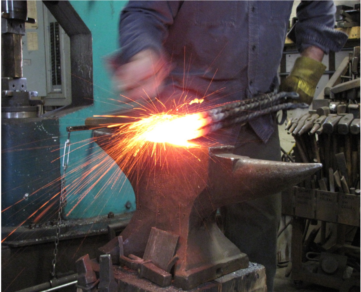
Brushing off the scale from the forge weld to keep the metal smooth and clean.
