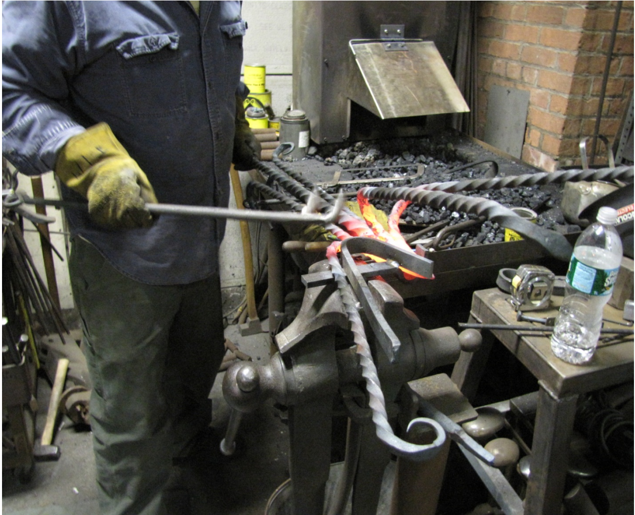
A jig was constructed to bend the arms all to the same curve. The arms were bent to this jig using a tool called a bending fork.
