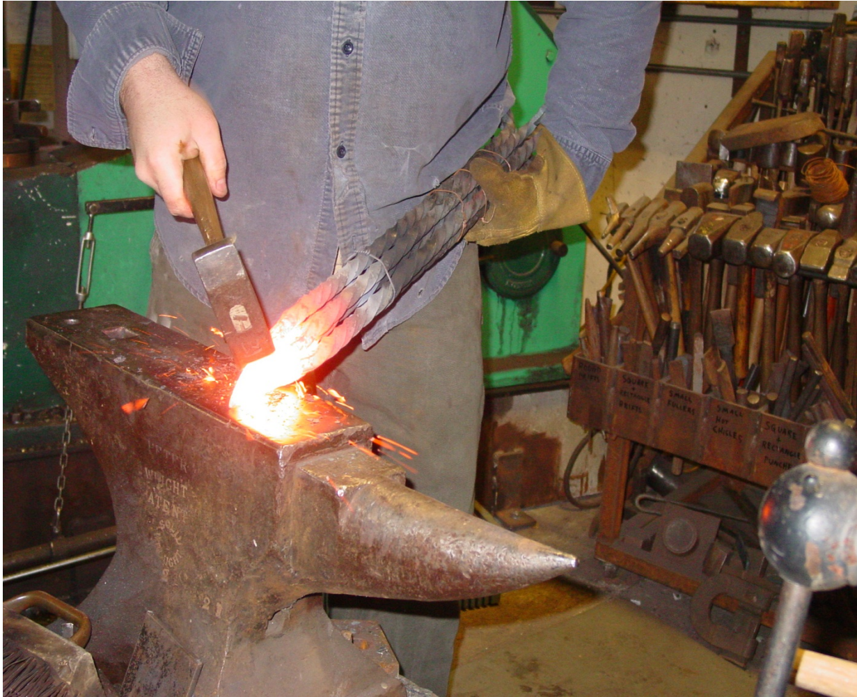
The bundle of arms, once heated to the proper temperature, are hammered together by the smith. This is called forge welding.
