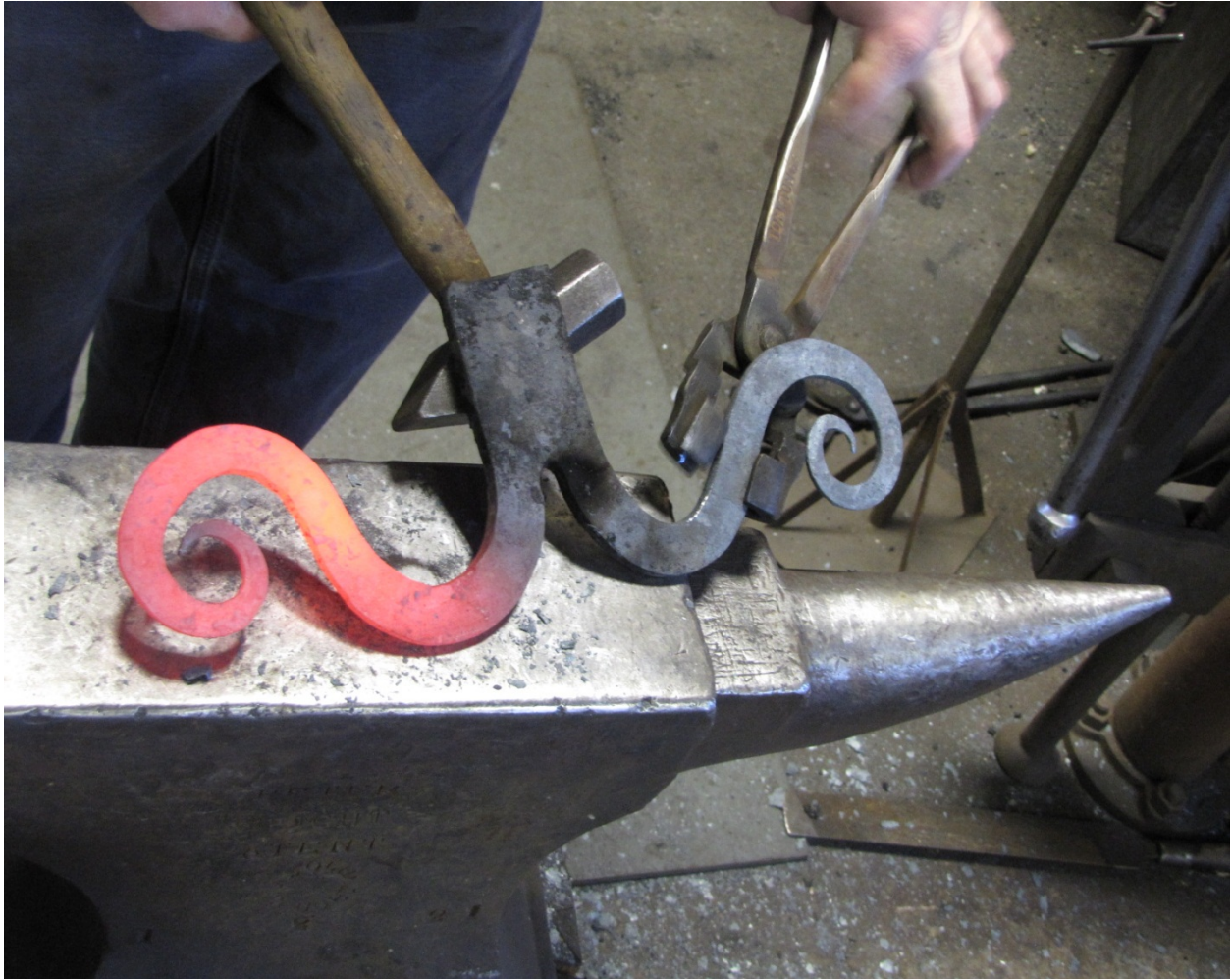
Checking the symmetry of the scroll by eye.
