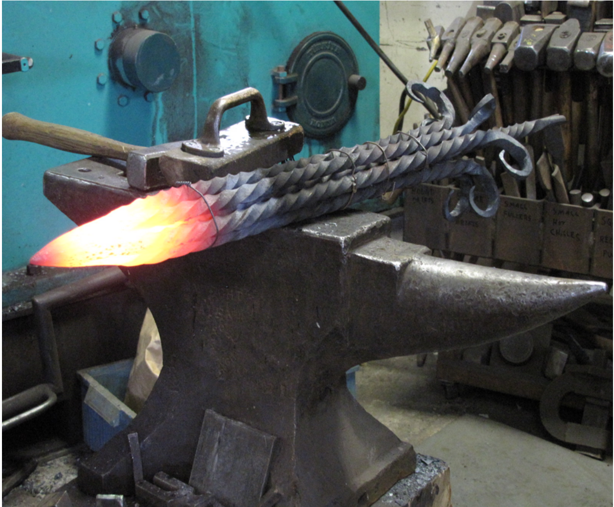
This is another view of the finished bundle weld showing the twisted arms that will be bent out to form the arms that will hold the candle cups.
