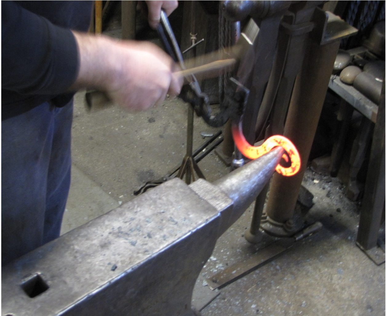
Using the horn of the anvil to adjust the spacing of the scroll to achieve the desired contour.
